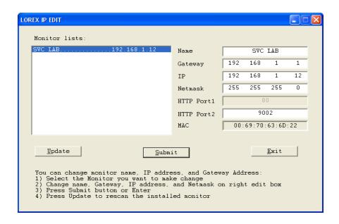
In order to use the Lorex technology Inc. DDNS service you must have signed up with the Lorex technology Inc. network in step 2 above. You will have received an e-mail providing you with the parameters to enter in this part of the setup.
